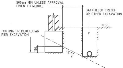
The installer shall undertake investigatory localised excavations near existing footings to ascertain their depth prior to excavating adjacent to them. It is noted that excavating to a depth below that indicated above shall not be undertaken without the written approval from a structural engineer.
